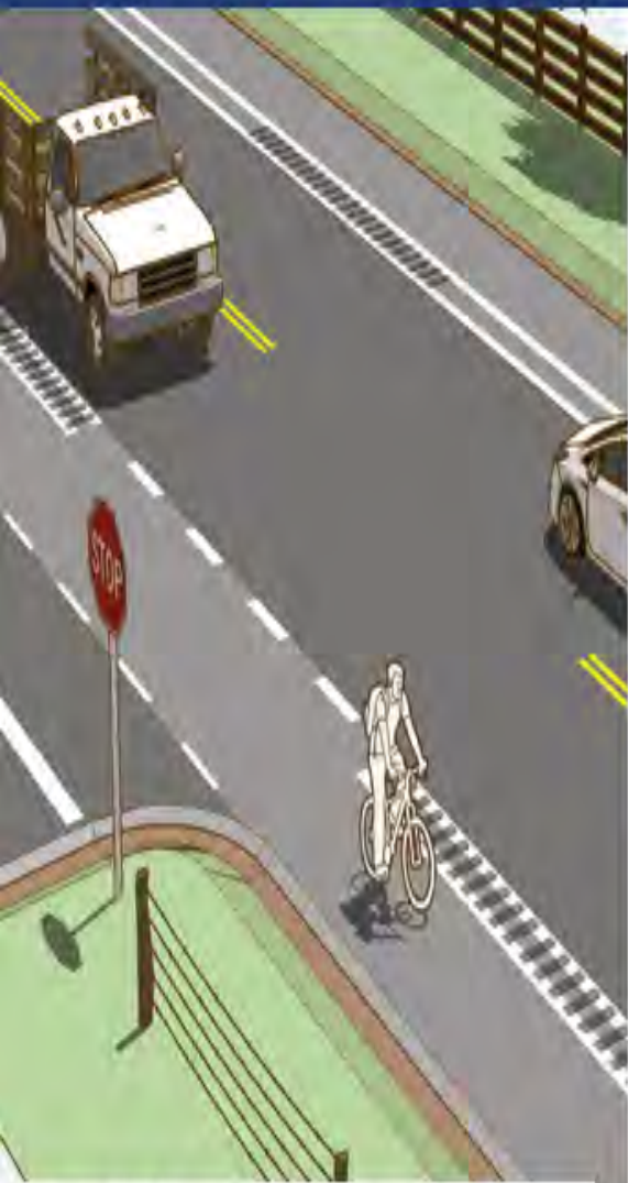
Figure 9. Example of a roadway reconfiguration using available roadway width to include bicycle lanes. Source: Rural Design Guide
