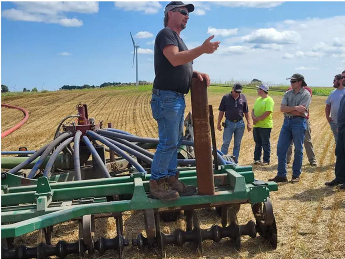
Dave Eisentraut of Eisentraut Ag Service in Waldo, Wisconsin, demonstrated his low-disturbance manure application system at the Oechsner Farm near Brownsville earlier this month during a Dodge County Field Day. The practice creates small, shallow slits in a recently harvested wheat field where manure from the pit at the Oechsner Dairy Farm is injected using a hose system Gloria Hafemeister/Special To Wisconsin State Farmer
