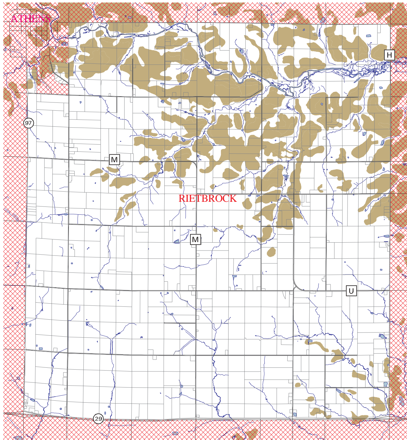
Figure 6-2 Suitable Soils-Septic Tank Absorption RIETSBROCK
